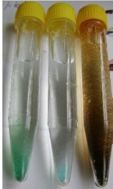
Figure 2: Results for tap water, 10 minutes, 24volts DC for three different electrodes Copper (left), Brass (middle), Iron (right) . Diameter of test tubes are 10mm.
