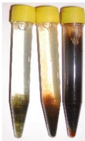
Figure 5: Filtered (left) tap (middle) and fish tank (right). Results after settling (vertical) for about 10 mins
