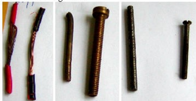
Figure 1: Electrodes used in experiment, copper left (wiring), brass middle (rod and bolt) and iron right, (threaded rod and screw). Approximate diameter of electrodes 2mm.
